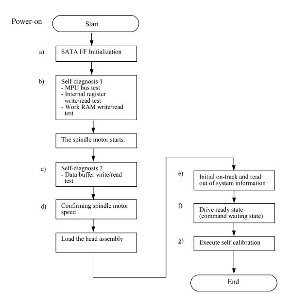
Figure 4.3 Power-on operation sequence
